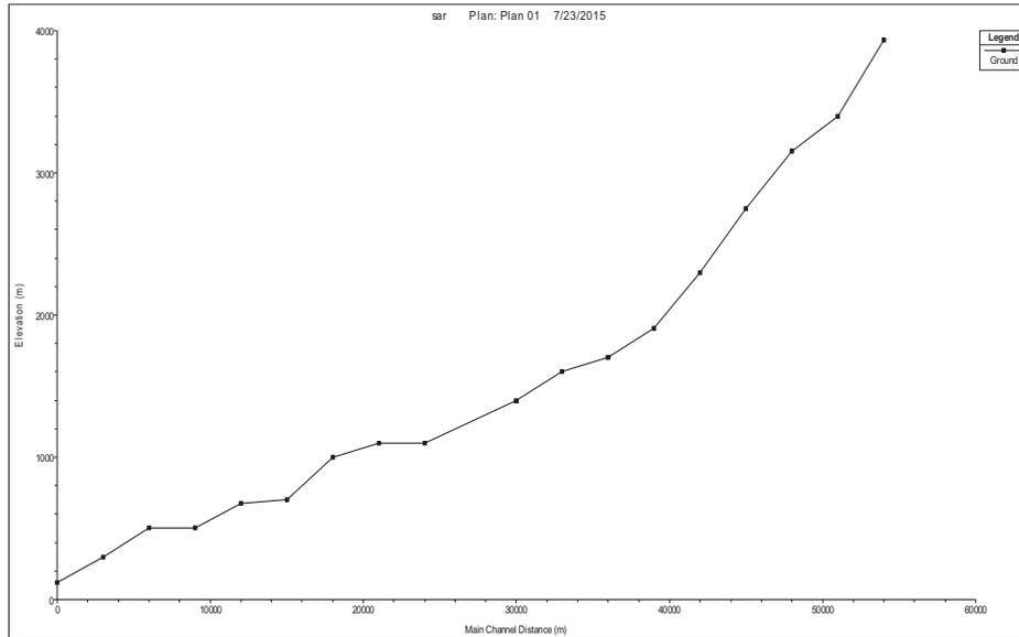
Fig. 2: Longitudinal profile of Sardabrud River
