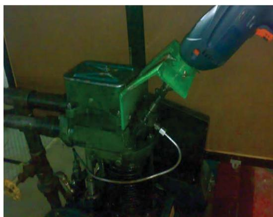
Fig. 4.2: Photographic View of Engine with Rotating Injector
