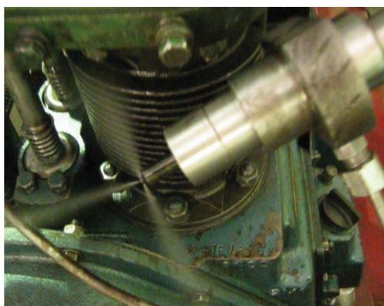
Fig. 5.1: Photographic View of Spray Pattern of the Conventional Injection
