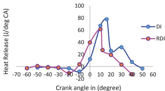
Fig. 6.7: Heat Release Rate
