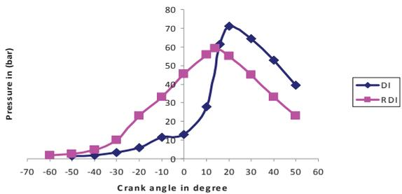
Fig. 6.6: Pressure-Crank Angle Diagram
