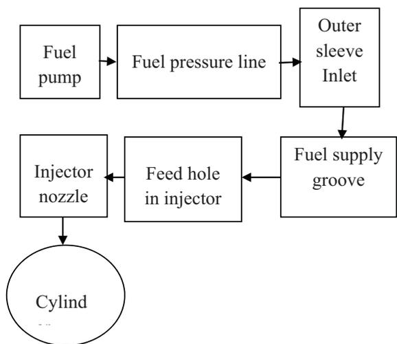
Fig 4.1: Fuel Flow Path Diagram
